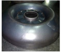
of the Rim. Tata Steel Limited has developed a new CRM Sheet and IDTR – Jamshedpur provided the Tooling Solution through which the Rim will be formed in 03 forming operations. It will increase the Productivity by 25% of the Automobile Vendors (MSME Sector).
